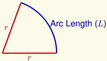
$$\text{Perimeter} = (\text{Arc Length}) + (\text{Radius}) + (\text{Radius}) = L + 2r$$
